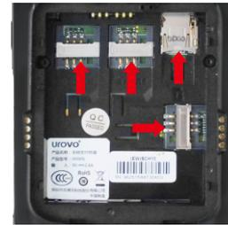
Insert the SIM/TF Card into their corresponding slots in the battery compartment.
