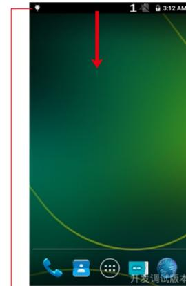
Tap the top of the screen, drag downwards and the USB setting interface will appear.
