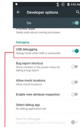
Check the USB debug if you intend to develop software and step through your code with the device.
